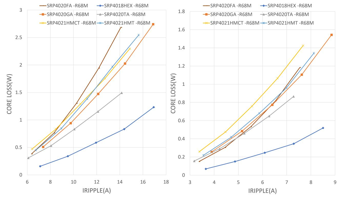
Fig. 5 Fig. 6. Measured core loss of different inductors at different I ripple values when the operating frequency are 500kHZ &1000 kHz.
